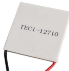
PT12715 CELULA PELTIER 12V 15A 180W 40x40 mm
