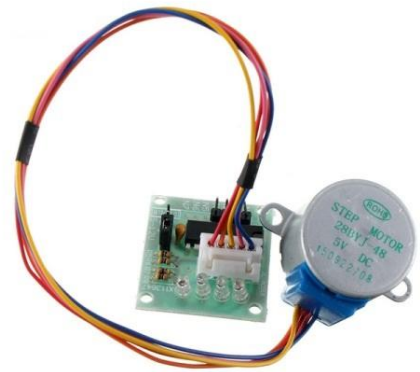
CP0096 MOTOS PASO A PASO + DRIVER ULN2003
