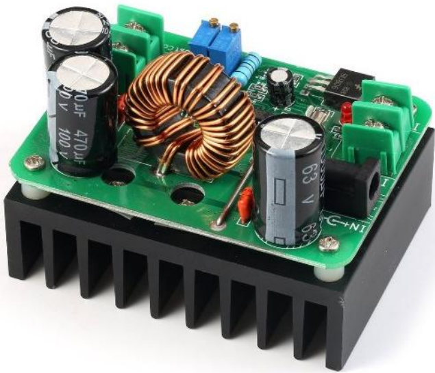
MD9013 MODULO STEP-UP 10-60 VDC A 10-80 VDC 600W
