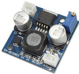
MD9004 MODULO STEP-DOWN 5A 4-48 VDC
