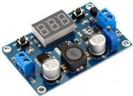
MD9007 MODULO STEP-DOWN 4.5 - 60 VDC 3A LM2596
