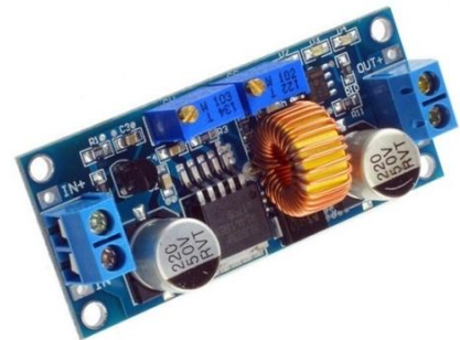
MD9008 MODULO STEP-DOWN 0.8 - 30 VDC 5A XL4015SA REG. TENSION/CORRIENTE
